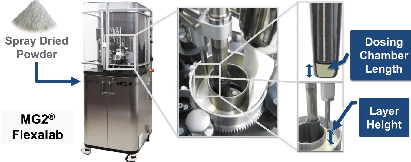
Figure 1 – MG2<sup>®</sup> Flexalab set-up: machine, rotary container and dosator.
