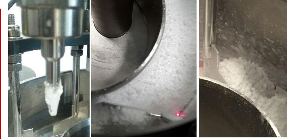
Figure 3 – Set-up and powder appearance before optimization.
